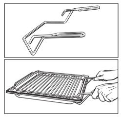
The handle makes it easier to take the tray and rack out of the oven, or to put them into it. The two prongs at the top go inside the tray or over the top of the rack and the U-shaped supports underneath
